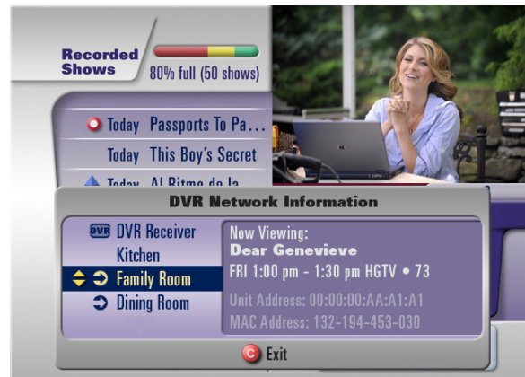
DVR Network Information on your primary DVR View networked set-top boxes in the home
